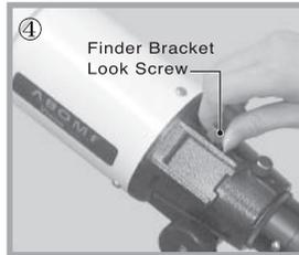
5. Attach the finder bracket as shown in the figure on the right. Tighten the finder bracket lock screw securely.
