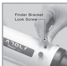
2. Attach the finder scope as shown in the figure. Tighten the finder bracket lock screw securely.
